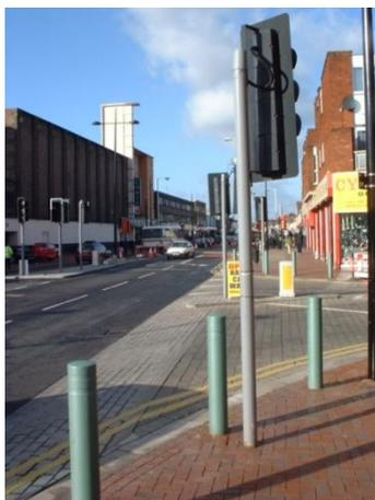
Figure 6 Bollards should be coordinated with other street furniture so an excess of poles isn't created - here the traffic signal could have been used to do the job of one bollard
