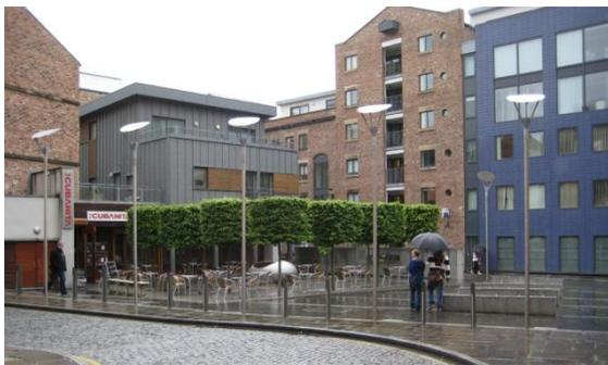
**Figure 13 Bollards used with lamp columns to enhance a pedestrian space**
