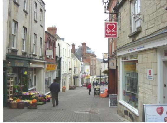
**Figure 14 Pedestrianised areas do not need long lines of bollards - service vehicles will use the centre of the space in any event**
