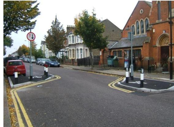
**Figure 2 Low budget traffic calming using plastic reflective bollards in an historic area**
